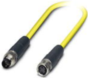
Sensor/Actuator cable, 3-position, PVC, yellow, shielded, Plug straight M8, on Socket straight M8, Cable length: 0.5 m
